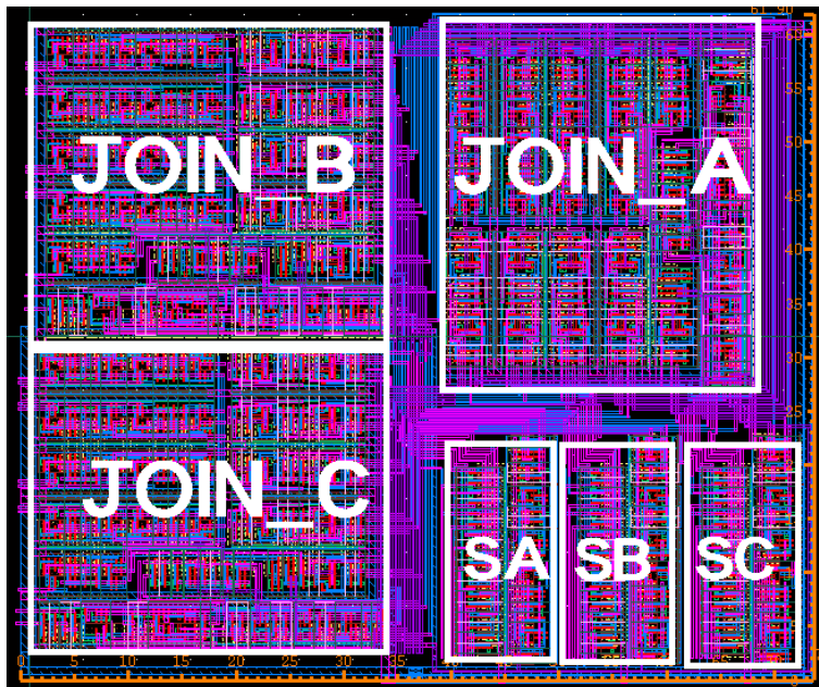
Figure 19: Layout of Async Router
