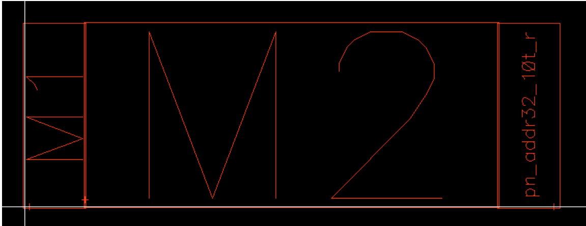
Figure 8: A 32x16 (32 word, 16 bits per word) dual-ported SRAM. Note that there are address decoders on both sides of the memory array M2.
