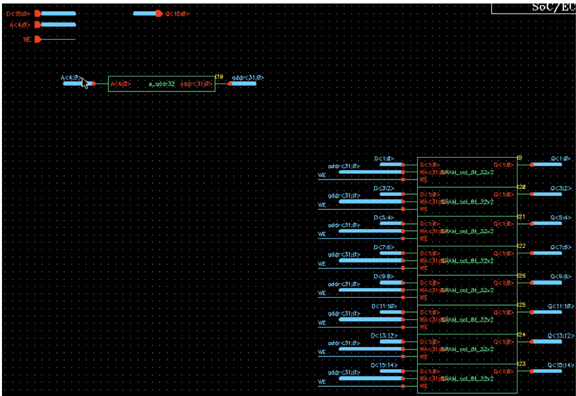
Figure 6: Schematic of 32x16 single-port SRAM. The interface is in the upper left. The address decoder (s_addr32 in this case) is below that. The SRAM columns are in the lower right. Note that because each column is two bits wide, there are 8 columns here that make up the 16 bits in each word.
