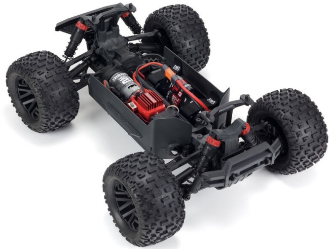
Fig. 3. Arrma Senton 4x4 V3 Mega 550 kit with the plastic top body removed used for the Kart [2].
