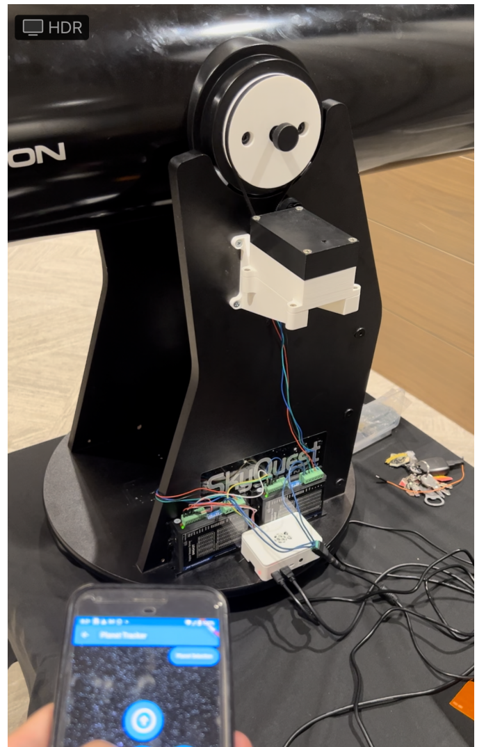
Fig. 11. The complete design of the telescope utilized during demo day.
