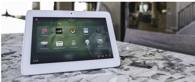
Fig. 2: Typical smart hub used to control various parts of the household. This one panel can control lighting, security, and AV systems. Provided by ValleyHomeTheatre.com
