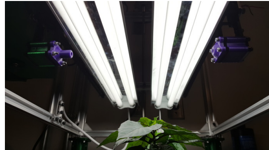
Fig. 10. A test of using a snoot to restrict light pollution produced by the grow light on the plant scanning system
