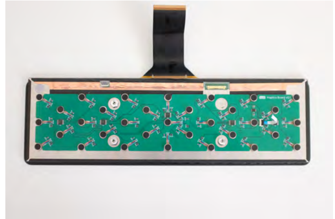
Fig. 13: Bottom view of the display assembly. Note that a haptics board has been applied.
