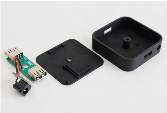
Fig. 16: Disassembly of the device bridge showing the power board, USB board, and enclosure.
