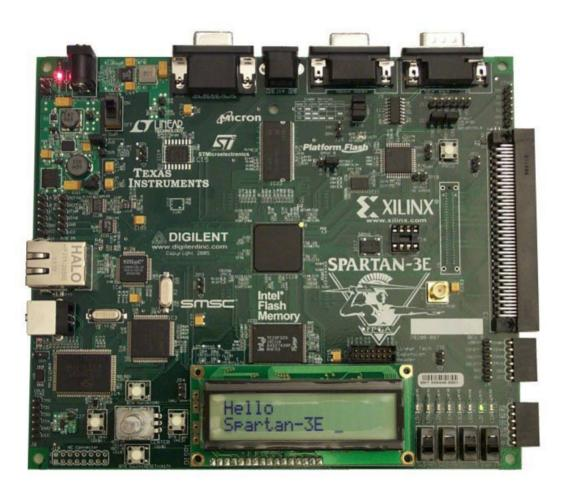
**FPGA:** Spartan-3E FPGA 500,000 gate equivalents, plus 40Kbytes of onboard RAM
