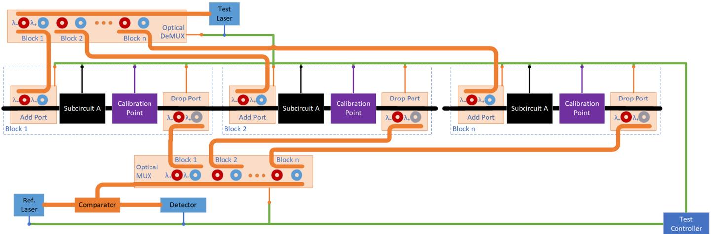
Fig. 6: DFTC Architecture details: Use of ring-resonators as test insertion and access points, use of separate normal mode ( $\lambda_0$ ) and test-mode wavelengths ( $\lambda_-, \lambda_+$ ), and a test controller to apply test inputs to compare DUT signals against a reference.
