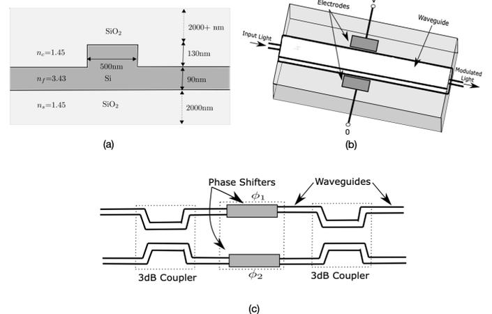
Fig. 1: SiP devices used in the DUT PICs: (a) SOI waveguide profile and the dimensions used;  $n_f = 3.43$  is the refractive index of *Si*,  $n_s, n_c = 1.45$  that of *SiO<sub>2</sub>*; (b) phase modulator; (c)  $2 \times 2$  MZI.
