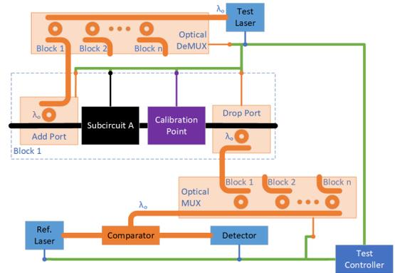
Fig. 5: Details of a DFTC block with RRs
