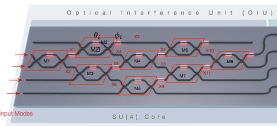
Fig. 8: SiP neural network subcircuit, borrowed from [2]. The MZIs are annotated  $\{M_1, \dots, M_8\}$  and the internal waveguides as  $\{X_1, \dots, X_{11}\}$ .
