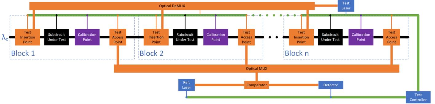
Fig. 4: SiP DFT and Calibration Architecture: Overview
