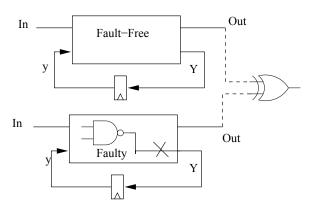
• Find a **sequence of inputs** (or input vectors) that produces an output 1 at the miter output, sometime in the future clock cycles
