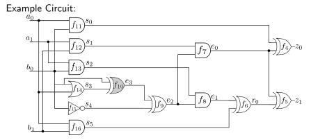
The circuit is buggy, bug = gate change at net  $e_3$ , which should have been an AND gate. Both outputs  $z_0, z_1$  affected by the bug.
