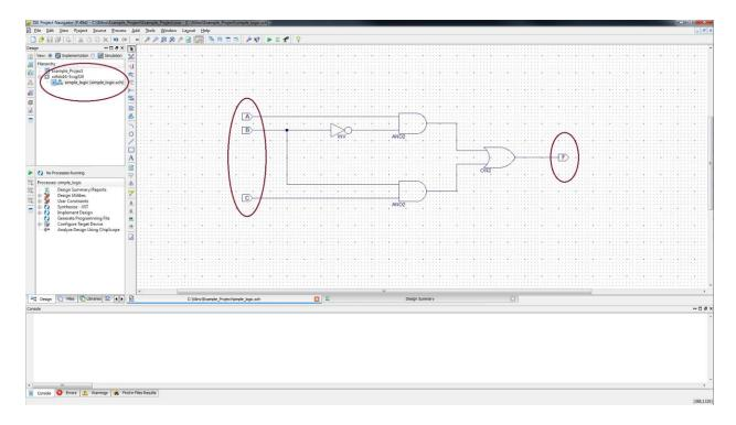
8. Now the resulting schematic looks like the following and it is ready for simulation or synthesis. Once your schematic is saved it should show up in the **Sources** pane in the upper left of the ISE screen.
