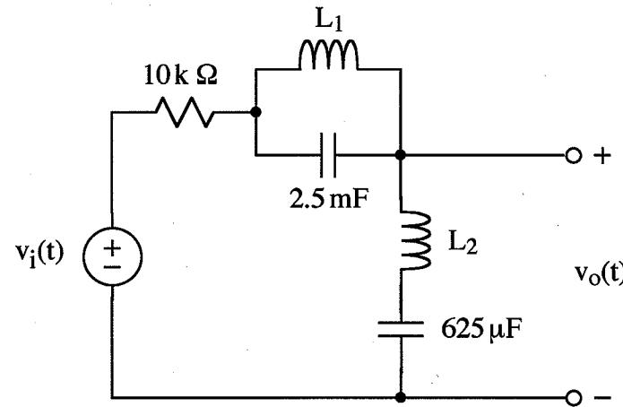
Find values of  $L_1$  and  $L_2$  for the above filter circuit such that the transfer function equals zero for the sixth harmonic and zero for the twelfth harmonic of periodic  $v_i(t)$  that has period  $T = 2\pi/60$  s.
