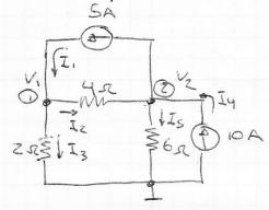
$$I_1 = I_2 + I_3 \longrightarrow 5 = \frac{V_1 - V_2}{4} + \frac{V_1}{2}$$
