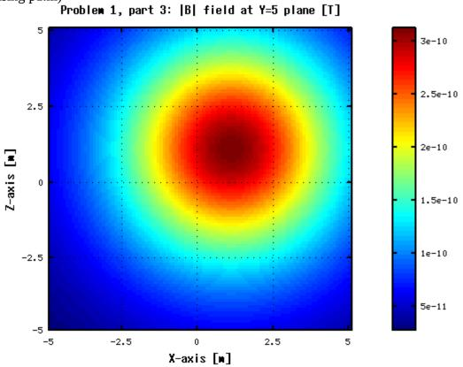
(optional) Code verification was done by solving the field generated by current circulating through a long wire analytically, and comparing it with the numerical solution (using verification.m). Plot below shows result:
