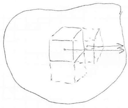
CONSIDER ANY DIRECTION, AND SINCE THE FACES OF THE SMALL CUBES ARE SHARED, THE FLUX THAT COMES OUT AT THE SURFACE OF THE BOUNDARY IS CONTRIBUTED JUST BY THE FACES 'DEFINING' THAT SURFACE.
