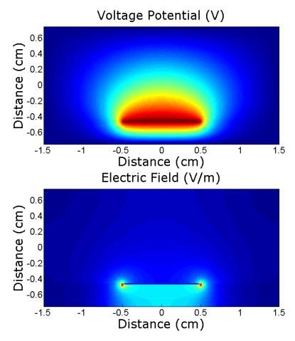
The analytically calculated impedance was 41.6  $\Omega$  while the simulated value came in at 38.0  $\Omega$ . Slightly better agreement can be achieved by using smaller grid spaces or by moving the boundaries further away. Of course, the trade-off is longer simulation time. The analytical computations also have buried assumptions that we are not necessarily aware of, making perfect agreement unlikely.
