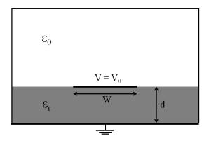
• Test your simulation under the conditions W = 1.0 cm, d = 3.0 mm, and  $\epsilon_r = 3$ . Use a value of V = 1.0 V for the potential of the top conductor. Use only Dirichlet boundaries of 0.0 V along the borders of the simulation domain. Choose a simulation boundary size and grid spacing that you think is appropriate in order to obtain accurate results. Plot the voltage and electric field distributions before calculating characteristic impedance.
