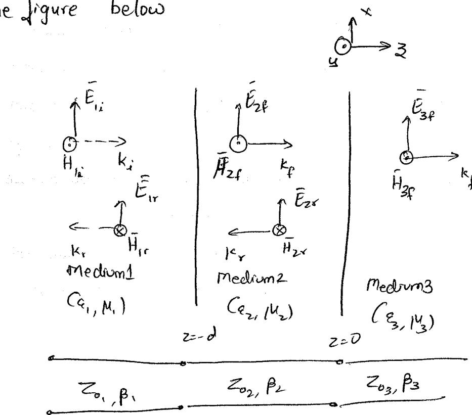
$\eta_1$ ,  $\eta_2$  and  $\eta_3$  are intrinsic impedance of the three medium and are separated by infinite planar boundary at  $z=-d$  and  $z=0$
