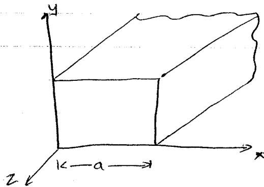
The waveguide is bounded in  $x$  &  $y$  directions and has its length along the  $z$  axis. Because the waveguide is bounded in the  $x$  and  $y$  directions, standing waves, represented by cosine and sine functions, have been chosen as solutions for  $f(x)$  &  $g(y)$  functions.
