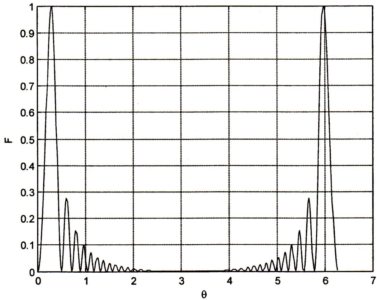
The polar plot of travelling wave antenna which is  $8\lambda$  is shown below:
