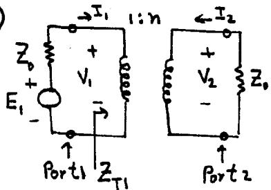
IN THE  $Z_0$  SYSTEM SHOWN, THE PARAMETERS  $S_{11}$  AND  $S_{21}$  ARE CALCULATED AS FOLLOWS:
