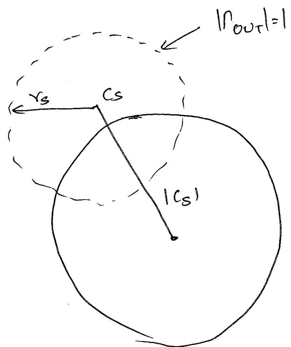
On one side of the stability  $\odot$  in the  $\Gamma_L$  plane we will have  $|\Gamma_{in}| < 1$  and on other side  $|\Gamma_{in}| > 1$ .
