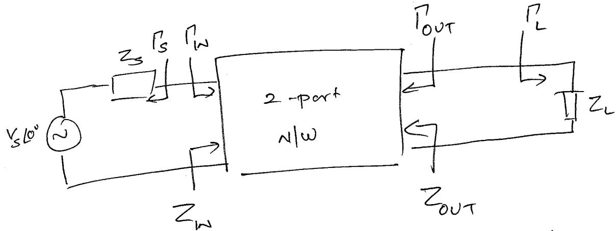
The two port N/w is said to be unconditionally stable at a given frequency if the real parts of  $Z_{IN}$  and  $Z_{OUT}$  are greater than zero for all passive load and source impedance.
