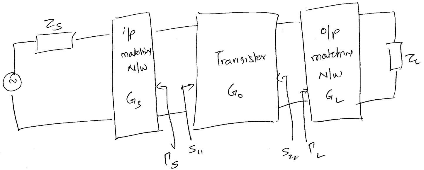
$G_{IS}, G_L$  - gain or loss produced by matching or mismatching between  ~~$P_S \& S_{11}$~~  i/p & o/p ckt.
