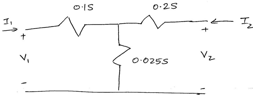
$$Y_{11} = \frac{I_1}{V_1} \Big|_{V_2=0}$$
