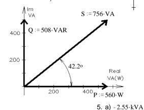
Draw a capacitor in parallel with load
