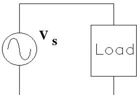
Assume the load consists of a resistor in series with a reactive component and the frequency is  $60\text{ Hz}$ .
