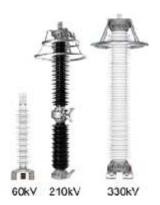
The insulation requirements of transmission lines are set by the peak voltage, but the power is determined by the RMS voltage. For sinusoidal waveforms the peak is 40% higher than the RMS. For DC they are both the same, so the RMS voltage can be 40% higher and the power can be twice as much for the same insulation. For each positive line there will also be a negative line with the same voltage magnitude so the neutral current can be zero.
