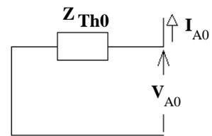
**Double line to ground fault**
