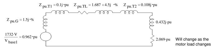
e) Calculate the currents and motor power when the motor in under full load.
