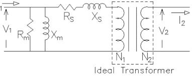
accounts for the no-load core power losses. These are due to the hysteresis in the B-H curve and to eddy-currents in the core. The series impedances,  $R_s$  and  $X_s$  account for winding resistance and leakage reactance. Both of these effects depend on the load current,  $I_2$ .
