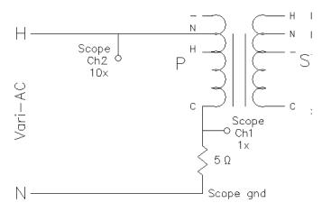
**common ground**, so make certain that the scope ground is connected to the neutral "N" side of the power. Unfortunately, that also means that we can't get a perfect voltage trace on Ch2. It will include a small error due to the  $5\Omega$  resistor, but because the resistor is small, we can live with it.
