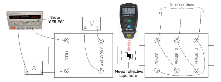
(above 1800rpm), hold the tachometer further away from the spinning coupling and/or check for more than one reflective tape on th couplings. Now that you have the DC motor spinning at a reasonably constant speed, you can get data to plot a curve like that shown in Figure 8-30 (p.398) of your textbook. You may wish to record the data directly into a spreadsheet to facilitate plotting the curve.
