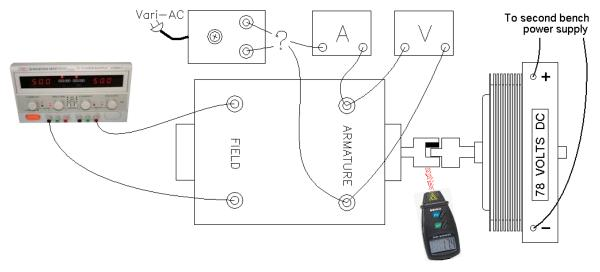
Set the armature voltage to 115V, or as close as you can get. Find the current knob on the Mastech power supply. Slowly turn it down until it begins to limit the current to the field and the motor rapidly accelerates – then immediately turn it back up again. Note that without field flux the motor speed can run away. Comment in your notebook. Say why someone should keep a hand on the Vari-AC's power switch from now on and why the armature supply should always be turned off before field supply.
