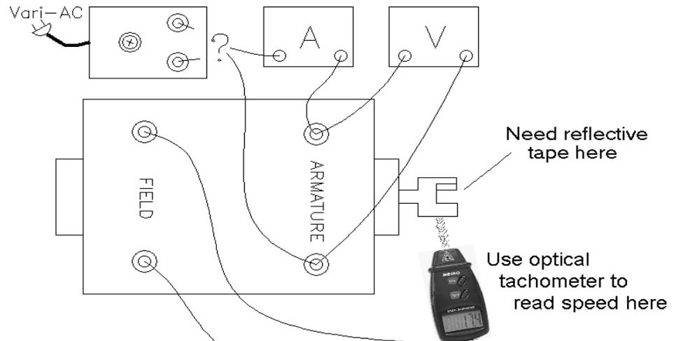
At an armature voltage of 50 V or less, briefly disconnect the field winding and observe what happens to the motor speed. (Note: If the motor doesn't speed up significantly, repeat with a higher armature voltage. Comment in your notebook.
