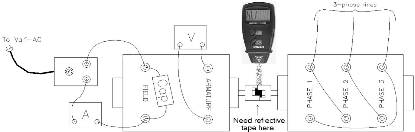
maximum. If the speed seems unreasonable high (above 1800rpm), hold the tachometer further away from the spinning coupling. Now that you have the DC motor spinning at a reasonably constant speed, you can get data to plot a curve like that shown in Figure 8-30 (p.398) of your textbook.
