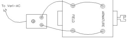
to use a shim under the DC motor to make the two line up well. Turn off the Vari-AC and plug it in. Plug the Rectifier box into the Vari-AC and hook the output to the DC motor. Polarity is not important. Switch on the Vari-AC and turn it up to make sure that you can drive the AC motor smoothly. Turn it back down.
