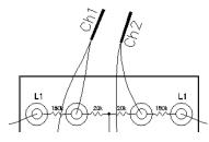
Move Ch1 & Ch2 so as to display a line phase and a generator phase on the scope at the same time. Set the speed of the DC motor so that the generated frequency is 60Hz. Set the field current so that the phase voltage magnitudes you see on the scope are the same. Try to ignore the higher-frequency "noise" on the generator voltage. Note the generator's field current (or voltage). Wait for the two
