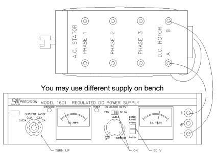
Turn off the 3-phase line breaker and hook up the 3-phase synchronous motor to the 3-phase lines (black, red, & blue) in  $\Delta$ . Pay no attention to the connector colors of the motor.
