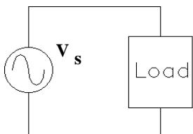
Assume the load consists of a resistor in series with a reactive component and the frequency is 60 Hz.
