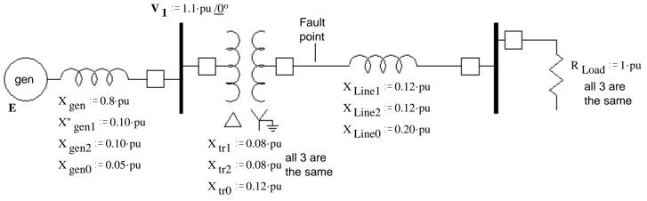
There is a phase-A single-line to ground (SLG) fault with a fault impedance of $\mathbf{Z}_{\mathbf{f}} := 0.15 \cdot pu$  $\underline{0}^{o}$ Find the fault current.You may be able to use some numbers already calculated in the example
