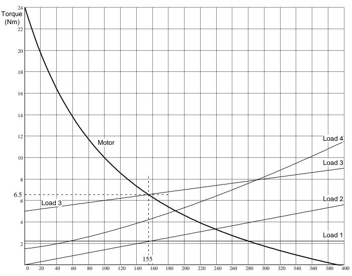
a) For each of the loads above, find the steady-state torque and speed if that load were connected to the motor. Show your work on the plot above and hand it in with your homework. I've found the answers for Load 3.
