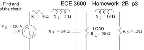
b) Use the Thevenin equivalent to find the current through the load resistor and the voltage across the load resistor.
