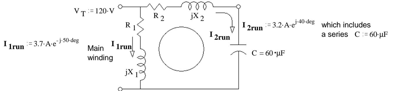
a) Find the run-speed impedances of winding 1 and winding 2 without the capacitor. Find both in rectangular form.
