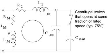
Now choose  $C_{run}$  to be ideal at normal operation and  $C_{run}$  +  $C_{start}$  to be ideal at startup.
