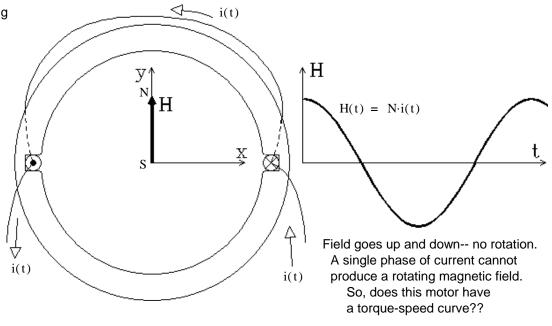
Yes it does. Think of the magnetic intensity vector, H, as being made up of two vectors half as large and rotating in opposite directions. The green (CCW) vector and the blue (CW) vectors shown below add up to be the H vector.
