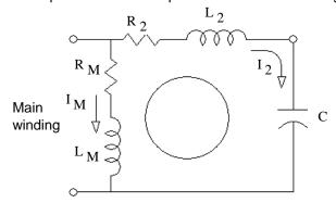
Ideally, choose a capacitor so that the current through the second winding (I<sub>2</sub>) leads the current through the main winding (I<sub>M</sub>) by 90°. Unfortunately, that will only be possible at one motor speed (or slip).
