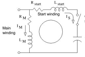
Centrifugal switch that opens at some fraction of rated speed (typ. 75%)
