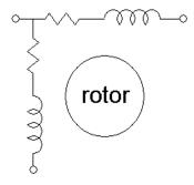
A better, but more complex and expensive system. R 2 Centrifugal switch that opens at some fraction of rated speed (typ. 75%) C start
