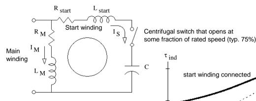
Ideally, choose a capacitor so that the current through the second winding  $(I_s)$  leads the current through the main winding  $(I_M)$  by 90° at startup (s = 1).
