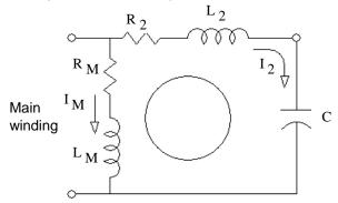
Ideally, choose a capacitor so that the current through the second winding ( $I_2$ ) leads the current through the main winding ( $I_M$ ) by 90°. Unfortunately, that will only be possible at one motor speed (or slip).
