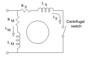
Start Direction: Reverse the leads to either of the windings to get the motor to start in the opposite direction.
