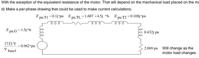
e) Calculate the currents and motor power when the motor in under full load
