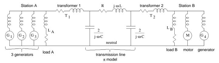
A T model of the transmission line may be easier to work with
