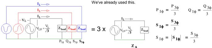
Anything not Y-connected can be converted to a Y- equivalent.  $Z_Y = \frac{Z_{\Delta}}{3}$
