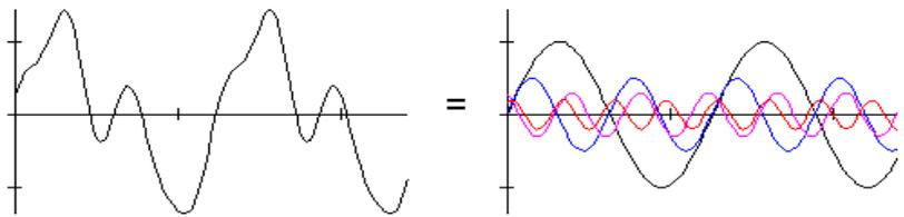
$V_{rms} = \sqrt{V_{rms1}^2 + V_{rms2}^2 + V_{rms3}^2 + V_{rms3}^2 + \dots}$
