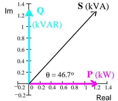
**Ex. 2** R & L together are the load. Find the real power P, the reactive power Q, the complex power S, the apparent power |S|, & the power factor pf. Draw phasor diagram for the power.
