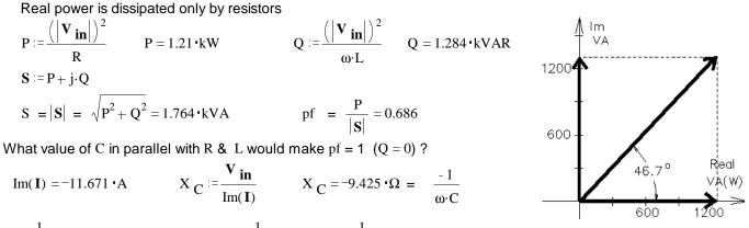
$$\frac{1}{|X_{C}| \cdot \omega} = 281 \cdot \mu F \qquad \text{OR..} \qquad \omega = \frac{1}{\sqrt{L \cdot C}} \qquad C := \frac{1}{L \cdot \omega^{2}} \qquad C = 281 \cdot \mu F$$
