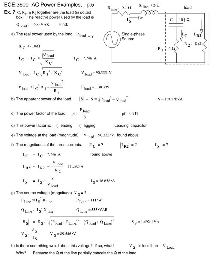
OR Partial resonance between the inductance in the line and the capacitance of the load.
