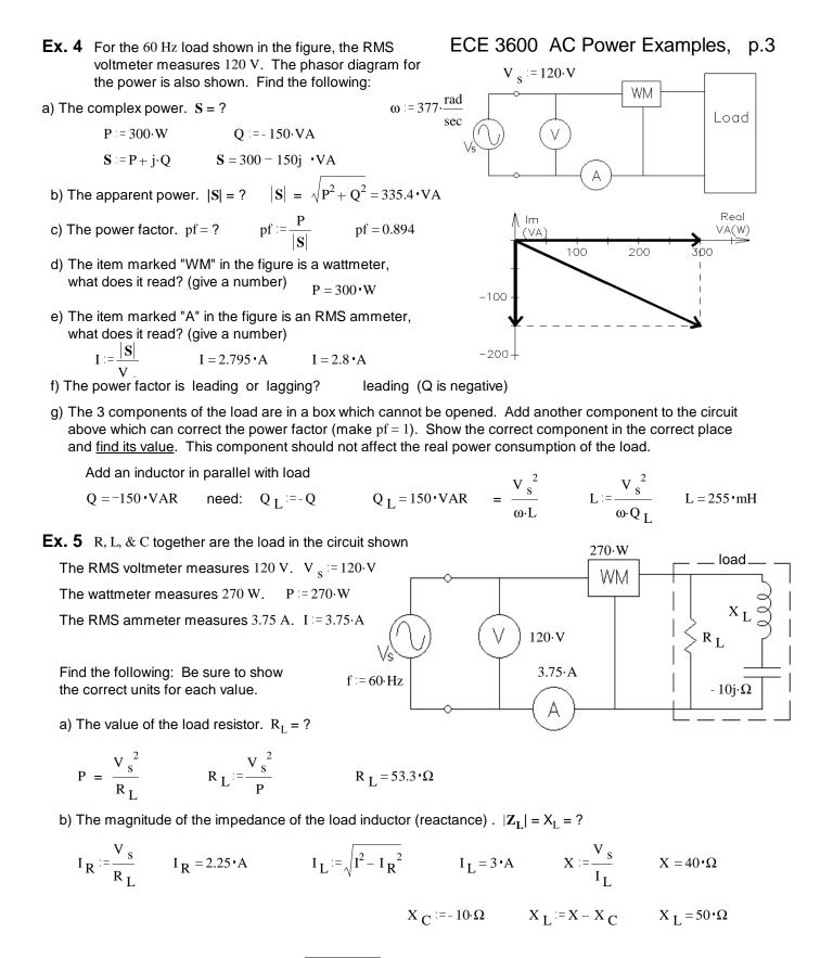
c) The reactive power. Q = ?  $Q := \sqrt{(V_s \cdot I)^2 - P^2}$  Q = 360 · VAR positive, because the load is primarily inductive
