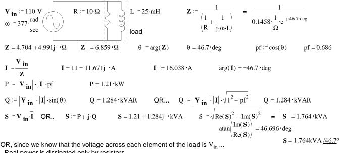
OR, since we know that the voltage across each element of the load is V<sub>in</sub> ... Real power is dissipated only by resistors
