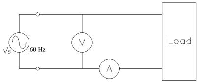
a) You add a capacitor, C, and the ammeter reading changes to 5.3A. Find the following:
