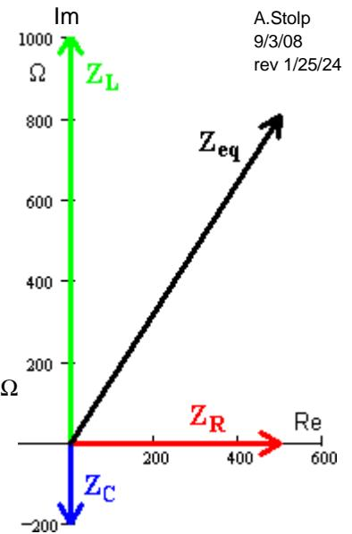
find the current:  $I := \frac{6 \cdot V \cdot e^{j0}}{Z_{\text{eq}}}$  magnitude:  $\frac{6 \cdot V}{948.5 \cdot \Omega} = 6.326 \cdot \text{mA}$  angle:  $0^\circ - 58.2^\circ = -58.2^\circ$   $I = 6.326 \text{ mA } / -58.2^\circ$
