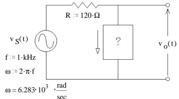
This can only happen if the angle of  $Z_{\text{box}}$  is positive, so  $Z_{\text{box}}$  is a inductor
