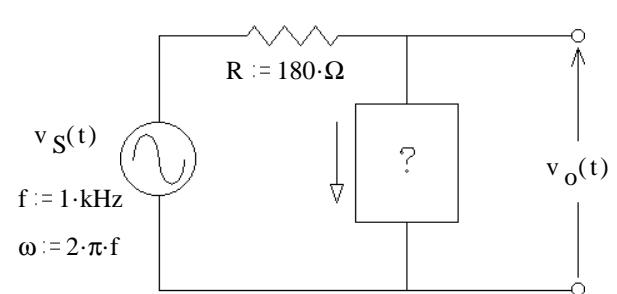
This can only happen if the angle of  $Z_{\text{box}}$  is negative, so  $Z_{\text{box}}$  is a capacitor
