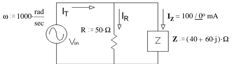
b) Find  $I_T$  in polar form.  $I_R := \frac{V_{in}}{R} = \frac{(4 + 6j) \cdot \text{V}}{50 \cdot \Omega} = \frac{4 \cdot \text{V}}{50 \cdot \Omega} + \frac{6j \cdot \text{V}}{50 \cdot \Omega} = 80 + 120j \cdot \text{mA}$
