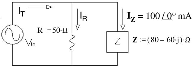
b) Find  $I_T$  in polar form.  $I_R := \frac{V_{in}}{R} = \frac{10 \text{ V}}{50 \Omega} \angle -36.9^\circ = \frac{10 \text{ V}}{50 \Omega} \cdot \cos(-36.9^\circ) + j \cdot \frac{10 \text{ V}}{50 \Omega} \cdot \sin(-36.9^\circ) = 160 - 120j \text{ mA}$
