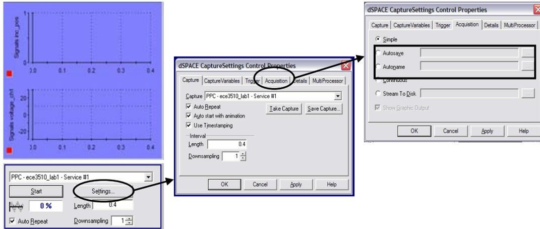
To save data outside dSpace the dialog progression for Figure 4 should be followed. The ultimate goal is to store the data graphed in the plot window to a .mat file for analysis in Matlab.
