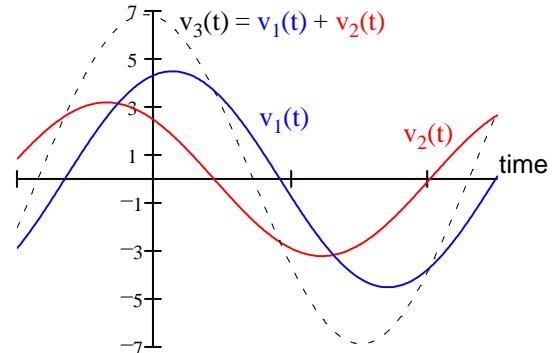
Phasors are based on cosines, so express  $v_2(t)$  as a cosine. Remember:  $\sin(\omega t) = \cos(\omega t - 90^\circ)$
