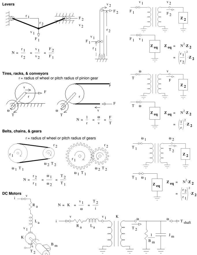
ECE 3510 Electrical Analogies of Mechanical Systems p.6
