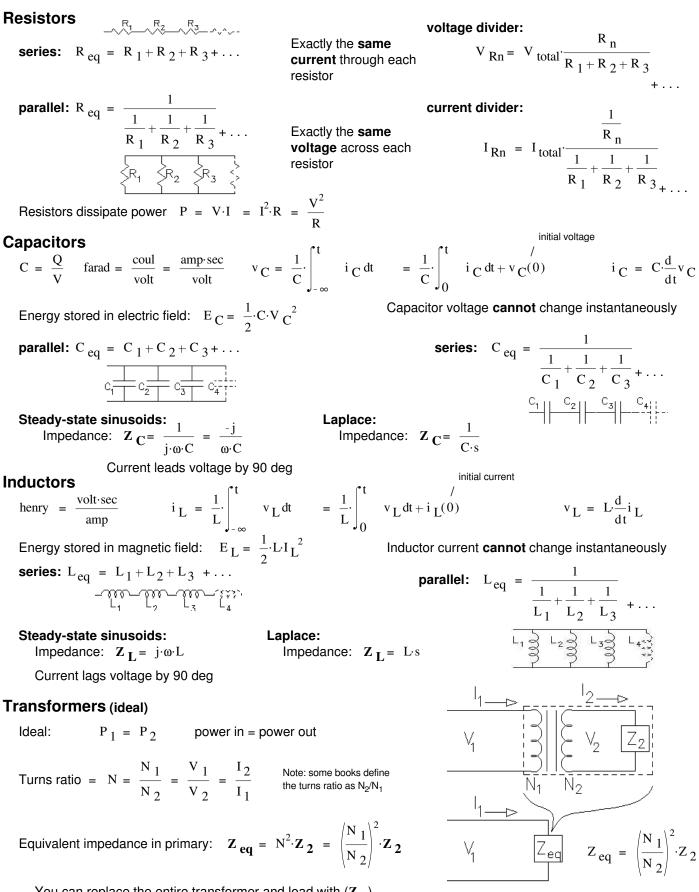
You can replace the entire transformer and load with  $(Z_{eq})$ . This "impedance transformation" can work across systems.
