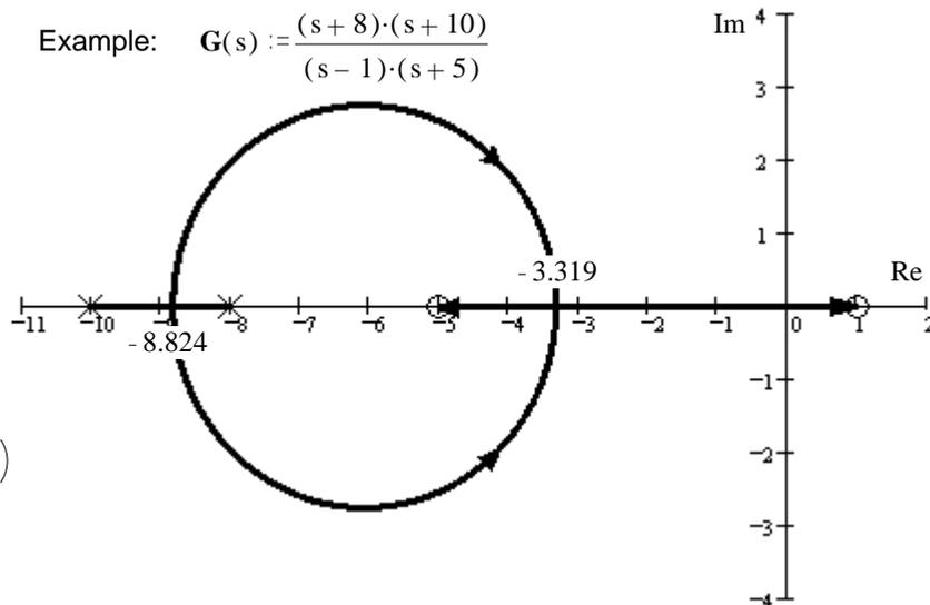
Breakaway (and arrival) points from the real axis ( $\sigma_b$ ) are also the solutions to:  $\frac{d}{ds} G(s) = 0$  where  $s$  is a real number (on the real axis)
