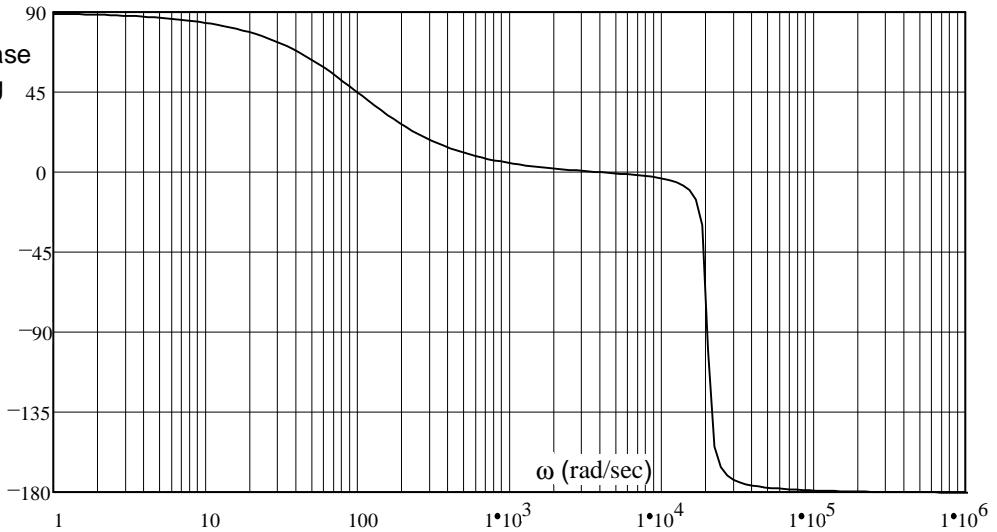
Note: A somewhat more involved method is outlined in Nise section 10.13 (p.660 in 3rd ed., 665 in 4th). That method involves estimating only one pole or zero at a time and then subtracting the effect from original to more clearly see the others. This can work much better with real experimental data. Real data always has delay effects and other non-linearities which make the process much harder.
